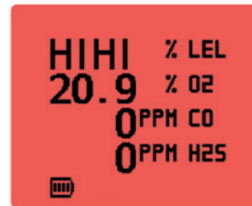
Red display in alarm conditions
